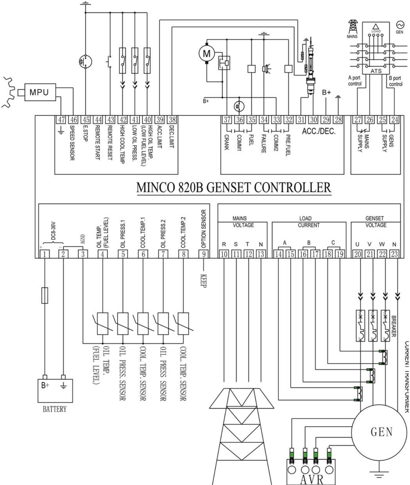
**Minco820B Outside wire connection drawing(Mechanical speed control)**
